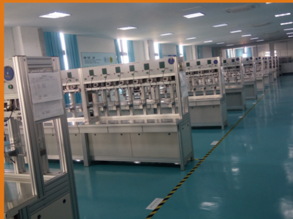
Gas meter constant temperature testing workshop
